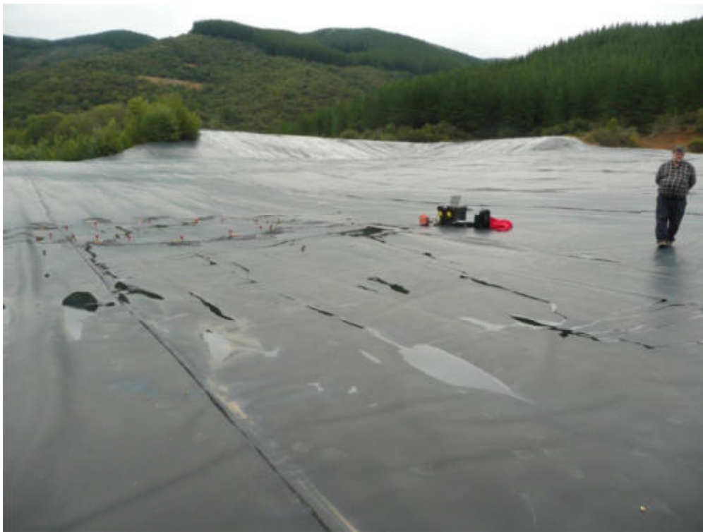
Figure 5.3 Shown is a 10-m circular array at location G5. Passive measurements were made of ambient noise from a generator, foot falls, etc.
