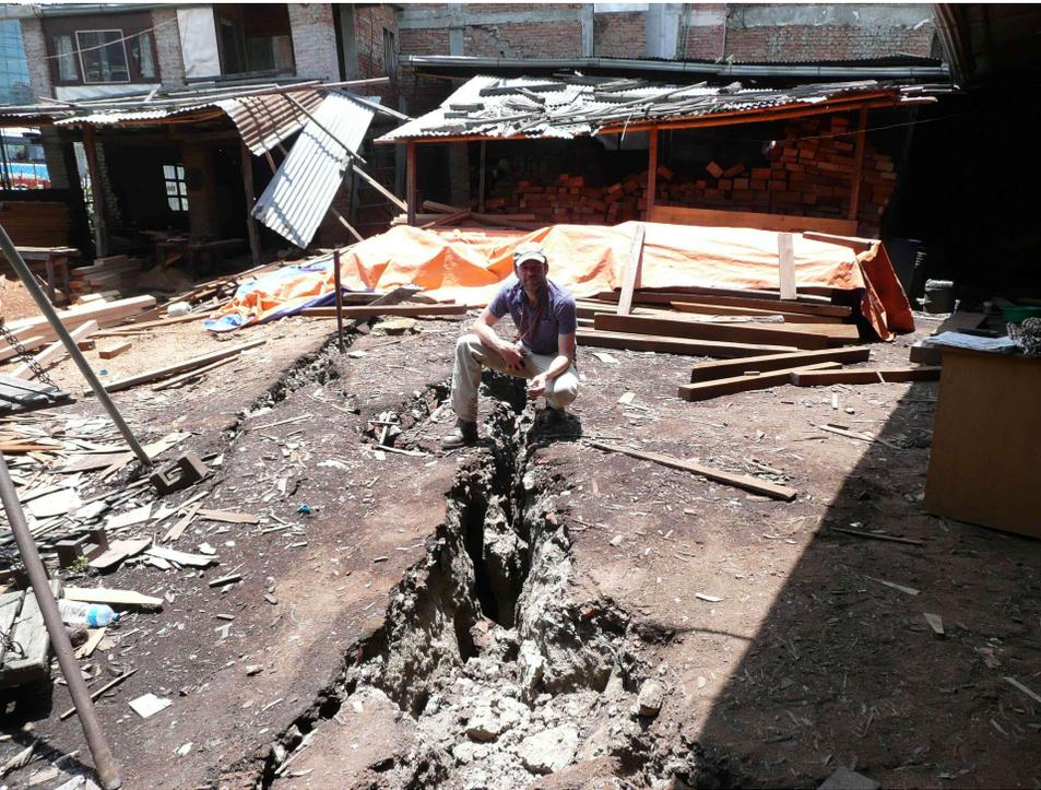
Cyclic failure of sensitive clays in Nepal 2015
