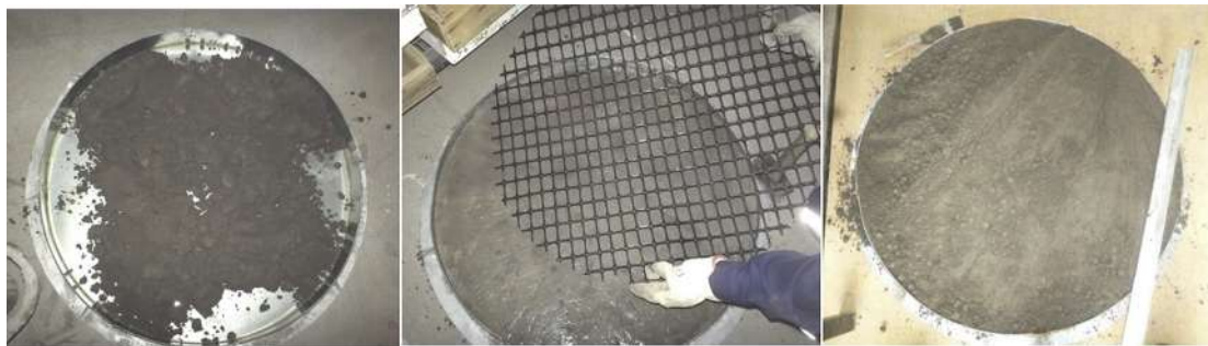
Fig. 6. Fabrication of test specimen with geogrid.
