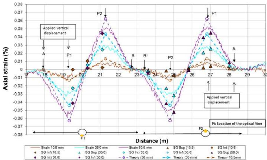
Fig. 7. Comparisons net strain measurements test Type IV.
