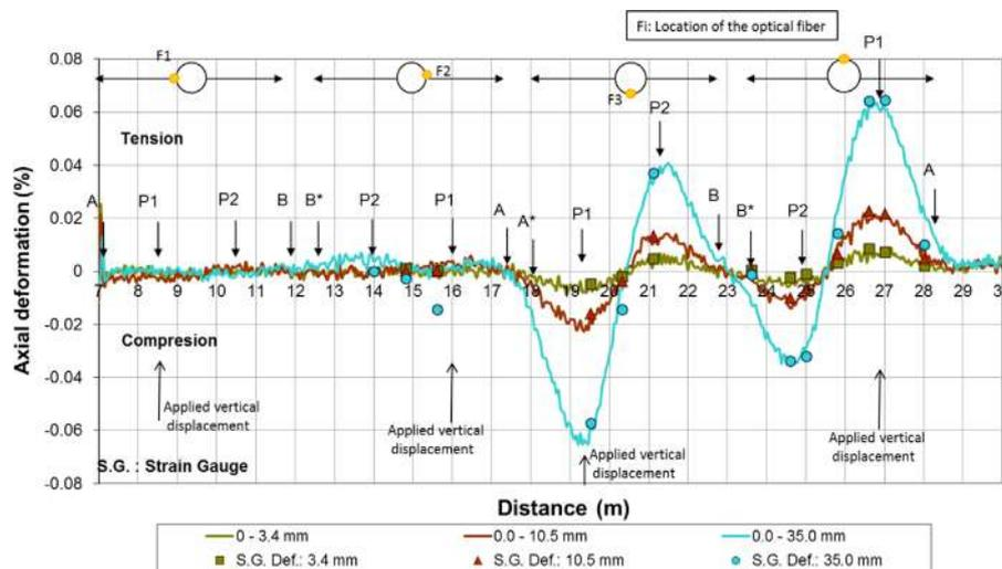
Fig. 4. Comparisons net strain measurements test Type I.
