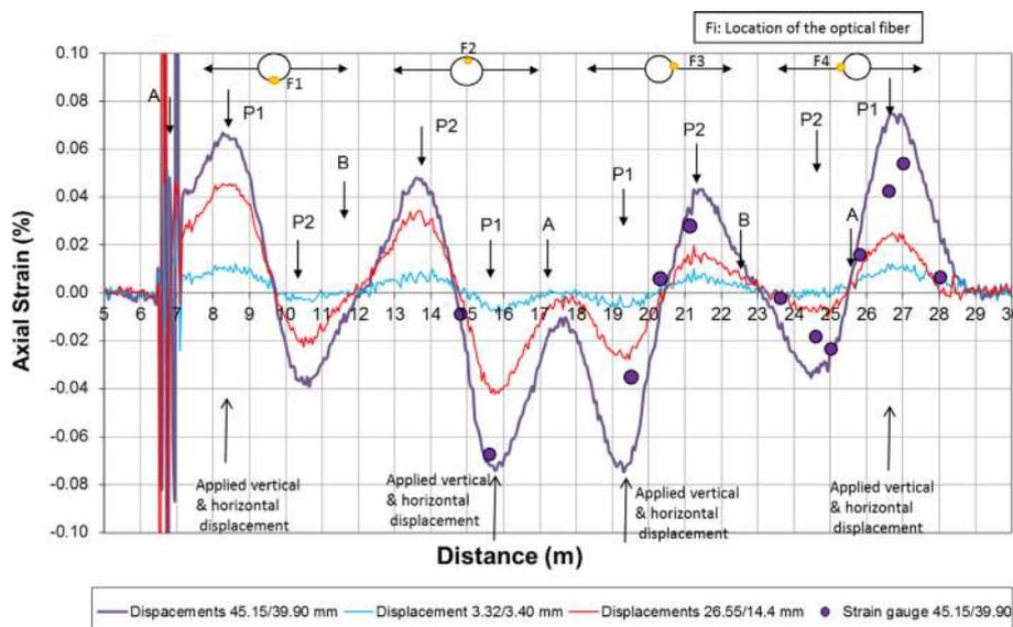
Fig. 5. Comparisons net strain measurements test Type II.
