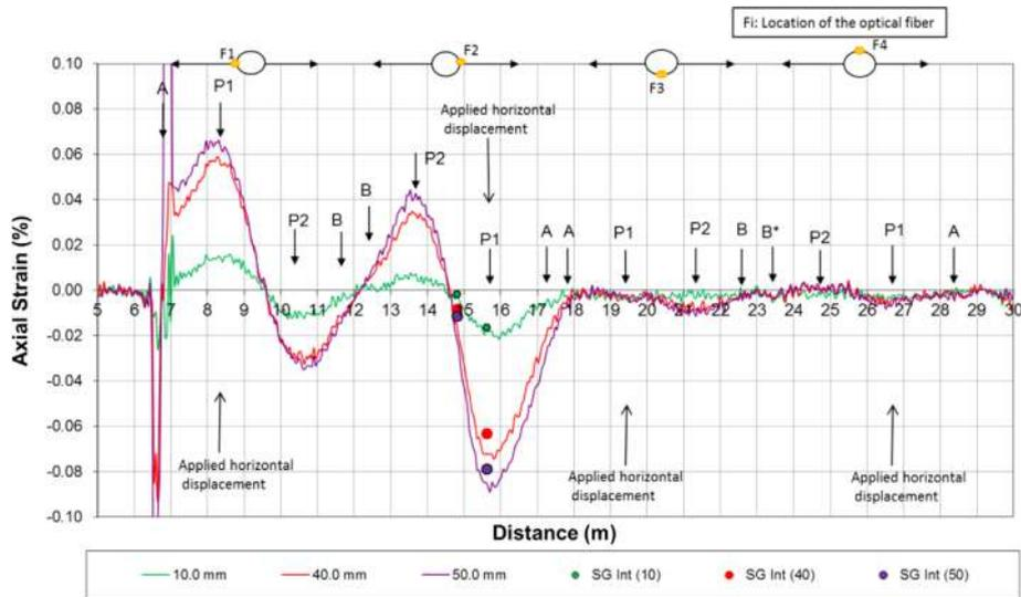
Fig. 6. Comparisons net strain measurements test Type III.
