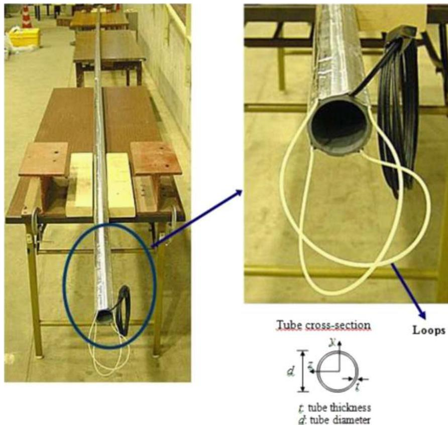
Fig. 1. PVC tube instrumented with optical fiber.
