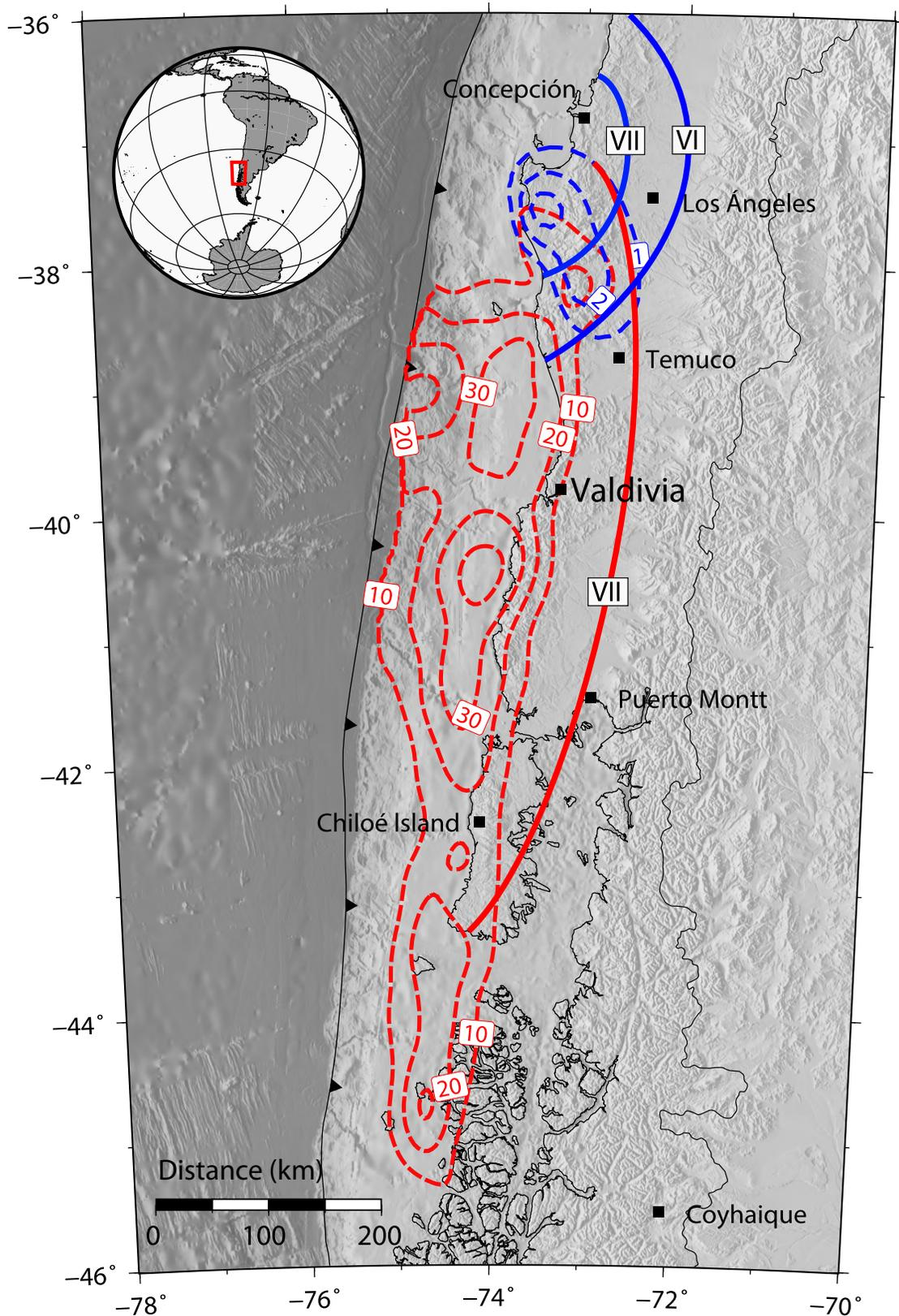
**Figure 1.** The 1960 Chilean earthquakes in central-south Chile. Segmented lines are iso-contours corresponding to the slip (in meters) of the 21 May  $M_w$  8.1 Concepción earthquake (blue) and the 22 May  $M_w$  9.5 Valdivia earthquake (red). Continuous lines are the Medvedev–Sponheuer–Karnik isoseismal intensities
