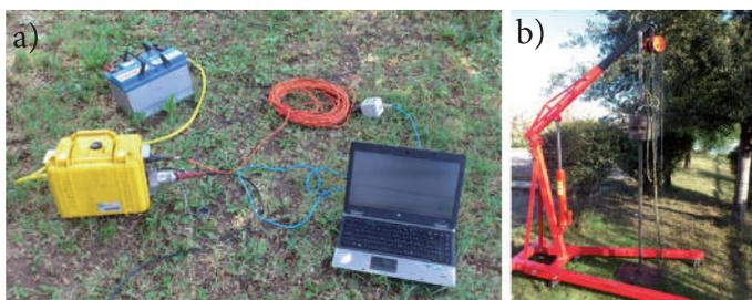
Figure 3: MASW field setup, a) seismograph, laptop and peripherals and b) impact load
