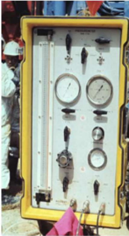
Figure 5.18. Photos of Pressuremeter Equipment, including Menard-type pressure panel, SBP probe, SBP cutter teeth, hydraulic jack, and monocell-type probe.
